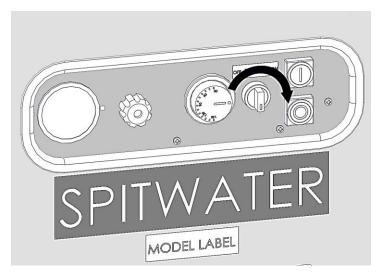
2. Turn the temperature adjustment knob to achieve desire cleaning temperature.
